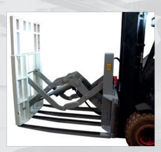
hand, saving a tremendous amount of time and labor expense. The Load Pusher is designed for heavy use under harsh conditions. Nonslipsheeted goods can be pushed into position with considerable force against other loads in order to create straight positioning and optimize space inside sea containers.
